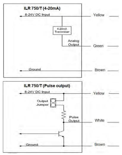
Figure 18: ILR 750 / 750T wiring
