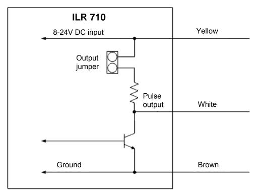
Figure 13: ILR 710 wiring
