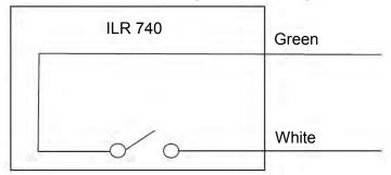
Figure 17: ILR 740 wiring
