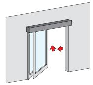
ONE SLIDING WING ONE FIXED WITH FULL EMERGENCY OPENING DEVICE
