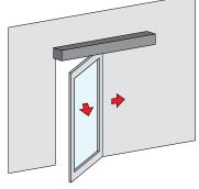
ONE SLIDING WING WITH EMERGENCY OPENING DEVICE ON A MOBILE WING
