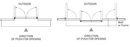
**WARNING**: In configurations where mobile wings equipped with ASM-N are joined to semi-fixed wings also equipped with emergency opening devices (full emergency opening device), it is necessary to fix the wings using the fittings supplied in the special set (optional).
