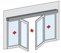
TWO SLIDING WINGS TWO FIXED WINGS WITH EMERGENCY OPENING DEVICE ON MOBILE WINGS
