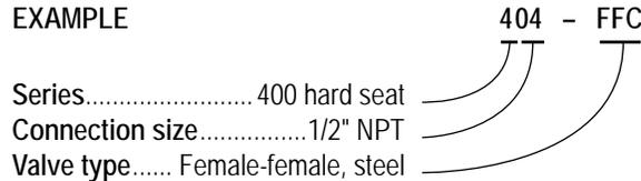
To meet all of your specific application requirements, the following additional options are available for these needle valves. To order all or any of these options, simply add them to the part number as shown in the diagram below.
