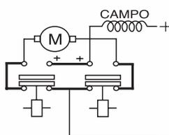
The lines ——— represent the links supplied with the motor reverser.
