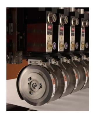
operations. The Performance Series Knifeholder is available in three sizes to accommodate shear, crush or razor slitting of just about any material. These advanced knifeholders also feature a unique 180 degree reversible blade cartridge, allowing use of both sides of the anvil blade and extending blade life.
