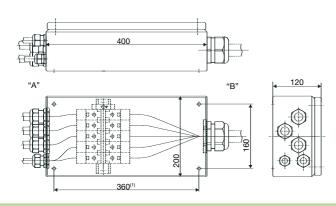
Electrical connection with customer supplied cable shoes. Clamping range 16-95 sqmm.
