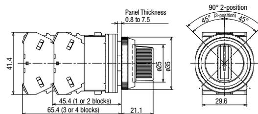
Terminal Screws: M3.5 Terminal cover: integrated
