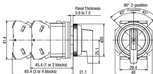
Terminal Screws: M3.5 Terminal cover: integrated
