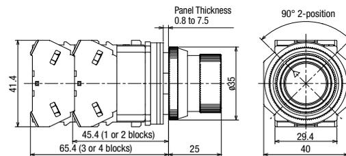
Terminal Screws: M3.5    Terminal cover: integrated
