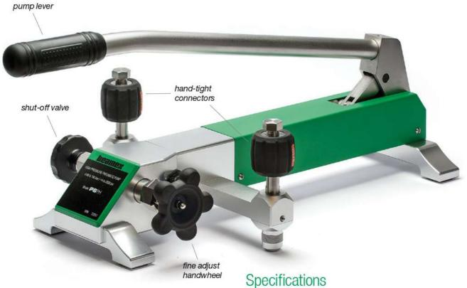
The PGPH is a hand-operated pneumatic (air as pressure medium) high-pressure table pressure generator. The pump is efficient in generating both vacuum and high pressure up to 140 bar (2,000 psi) quickly and effortlessly. It takes less than one minute to generate the maximum pressure. The PGPH is equipped with an adjustable volume control, providing excellent fine-tuning of generated pressure, and two hand-tight connectors allowing fast and easy connections without the need for any tools.
