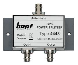
The power splitter is built in a HF-proof housing with an insulated base plate. The unit can therefore be easily screwed to the wall near the GPS receivers. The GPS antenna is connected to the BNC-connector called "Antenna In". On the opposite side of the housing two signal outputs to the GPS receivers are located.
