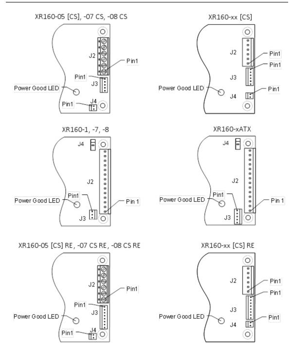
Figure 4-3 XR160 Output Connectors Layouts
