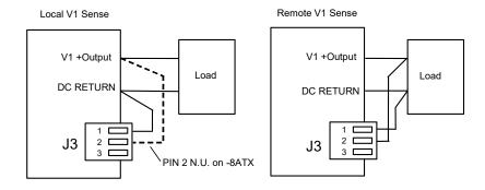
Figure 3-3 Remote V1 Sensing: XR160-1[ATX], -7[ATX], -8[ATX]
