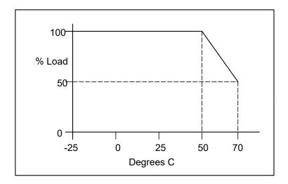
Figure 3-1 XR160 Output Power vs. Ambient Temperature Envelope
