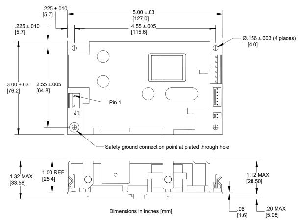
Note: Recommended standoff size is .375" high and all mounting hardware should be less than .28" in diameter. A standoff less than .375" high is acceptable when a thin insulator, 0.4mm thick (polyester, fish paper or equivalent UL rated 94V-2 minimum) is placed between the XR160 and the mounting chassis (refer to applicable UL standard for clearance requirements).
