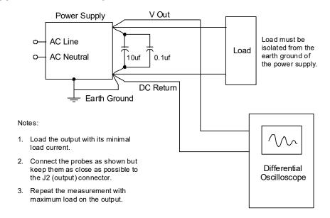
Figure 3-2 Ripple Noise Measurement Setup
