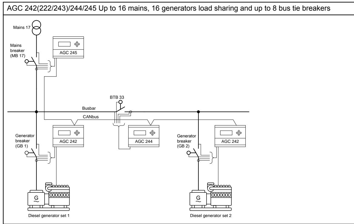
AGC 242(222/243)/244/246 Up to 16 mains with tie breakers, 16 generators load sharing and up to 8 bus tie breakers
