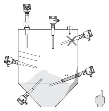
Horizontal installation/vertical installation
