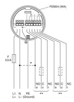
$U \approx 19 \ V \dots 253 \ V \ (AC) \qquad U = 19 \ V \dots 55 \ V \ (DC)$
