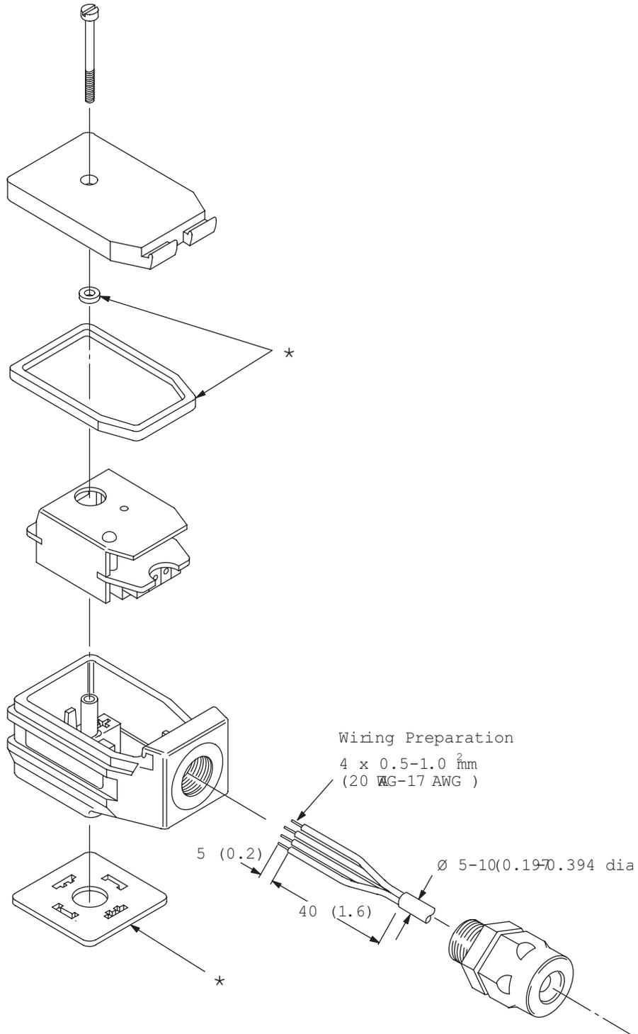
\*All seals must be fitted correctly at plug installation to provide protection to IP67 (IEC 529).
