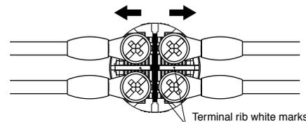
As shown in the illustration below, mount the live section cover so that the mounting legs of the cover engage with the concave parts of the main unit.
