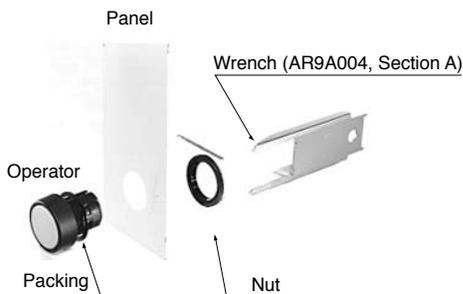
Note: Recommended tightening torque is from 1 to 1.5N·m
