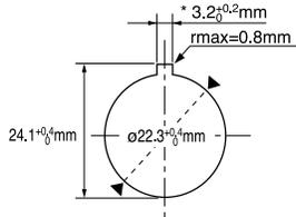
The switch mounted as a  $\phi 25\text{mm}$  diameter unit.
