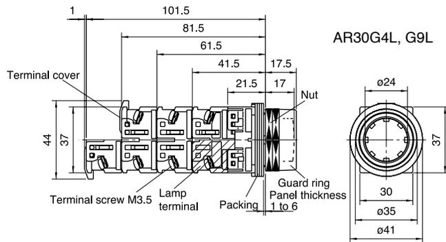
Extended with full guard (24mm dia. with openings)
