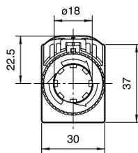
**Unibody push-lock, turn-reset (40mm dia.)**
