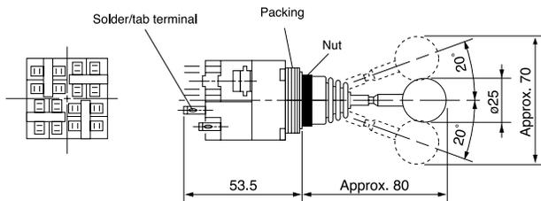
Notes \* The contact arrangement is operable in the designated direction by pulling the lock piece in the central position with the fingers. The lock piece will return automatically and locks when the lock piece is released in the central position. The lock piece locks in the central position only.
