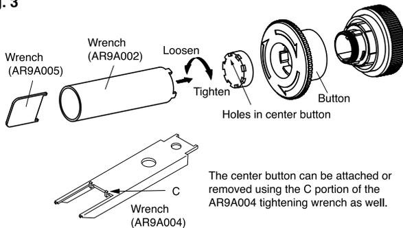
The center button can be attached or removed using the C portion of the AR9A004 tightening wrench as well.
