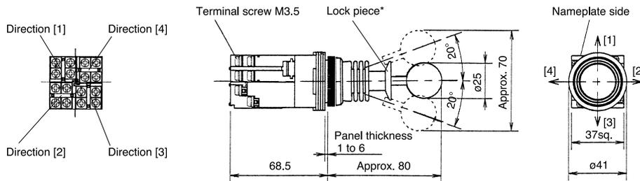
Notes \* The contact arrangement is operable in the designated direction by pulling the lock piece in the central position with the fingers. The lock piece will return automatically and locks when the lock piece is released in the central position. The lock piece locks in the central position only.
