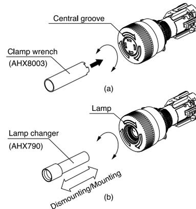
Note: The lamp and neon lamp are special models for the AR22VGF. Use only these special lamps for replacement.
