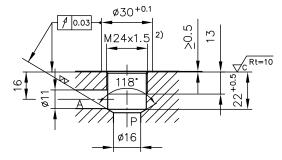
Counterbore  $0.5^{+0.2}$  (max.  $\varnothing 30^{+0.1}$ ), exclusively required for pressures at A in excess of 100 bar.
