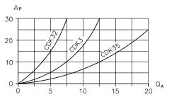
Q<sub>A</sub> Volumetric flow rate (lpm); ∆p Flow resistance (bar)
