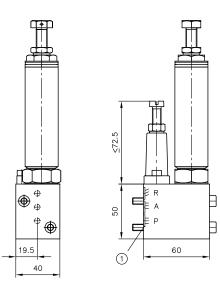
Sealing with O-rings 7.65x1.78 NBR 90 Sh
