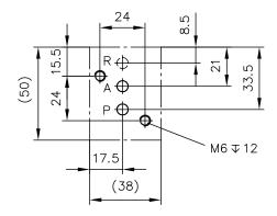
The hole pattern corresponds to that of type ADM 11 P as per  $\underline{D}$  7120. The 0-ring counterbore for the drain port R (or L) is present but is only required for type CDK..-SP.
