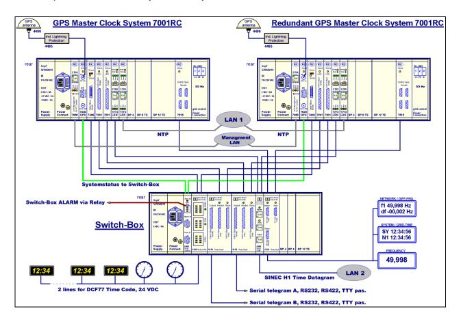
This system guarantees that the signal output always switches over to the redundant system as soon as the latter demonstrates a lower fault level than the master system.
