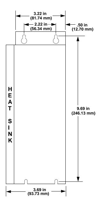
Figure 5-9: 500 W Standard Drive (non-DN) - Front
