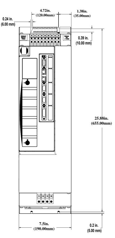
Figure 6-15: Size 4 460V Smart Drive - Front View
