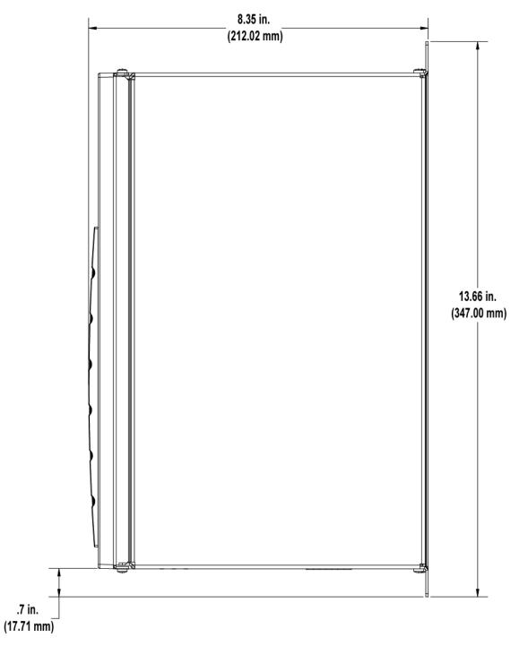
Figure 6-10: Size 1 460V Smart Drive - Side View
