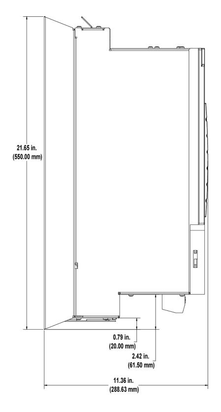
Figure 6-14: Size 3 460V Smart Drive - Side View
