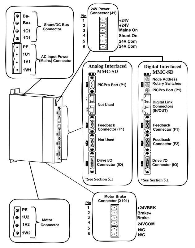
Figure 6-1: Connectors on the Size 1 460V Smart Drive
