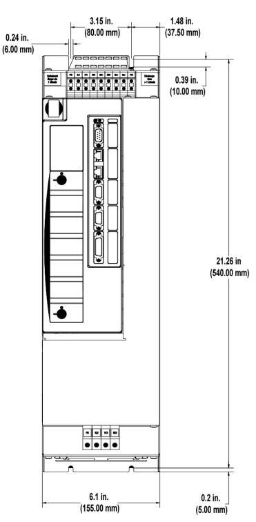
Figure 6-13: Size 3 460V Smart Drive - Front View
