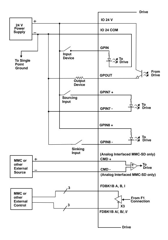
Figure 5-6: Wiring Diagram for Drive I/O Connector (IO)
