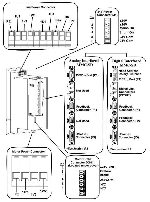
Figure 6-5: Connectors on the Size 3 460V Drive
