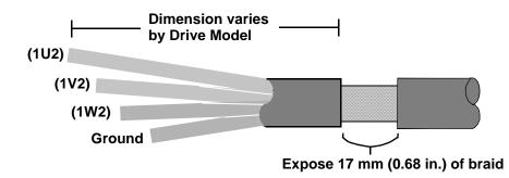
4. Attach the individual wires from the motor cable to their assigned terminal. Refer to Chapters 5 and 6 for front panel connectors and terminal assignments.
