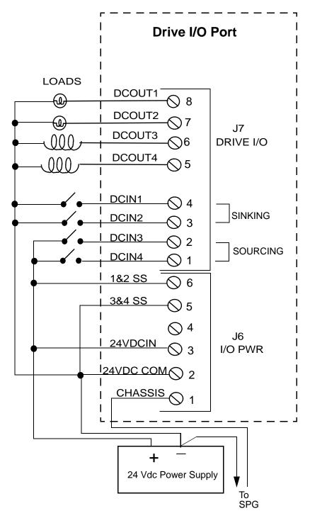
Figure 7-3: Connecting Devices to the Drive I/O Port
