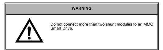
8.8.1 Connecting the 230V MMC Smart Drive to 300 W Shunt Module
