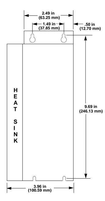
Figure 5-10: 1 kW & 2 kW Narrow Drive (-DN) - Front View
