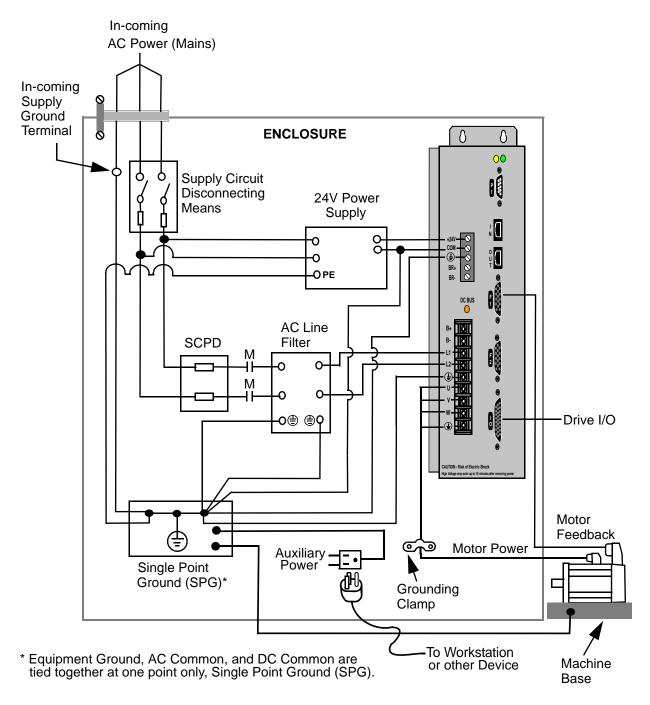
Mount the filter as close to the Drive as possible. If the distance exceeds 600 mm (2.0 ft), use shielded cable between the Drive and the filter, strapping the shield to chassis at each end of the cable. This is particularly important for attenuation of higher frequency emissions (5-30 MHz).
