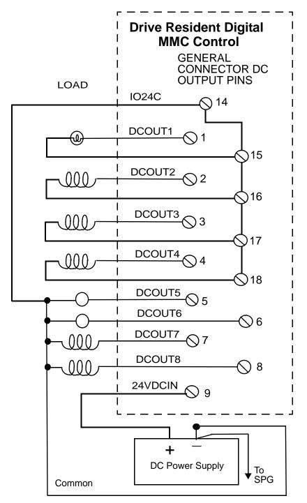
Figure 11-7: Connecting Output Devices to the General I/O Port (C5)
