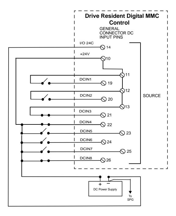
Figure 11-8: Connecting Input Devices to the General I/O Port (C5)
