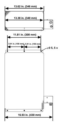
Figure 4-7: Mounting Dimensions for 460V External Shunt (P/N M.1302.7063)
