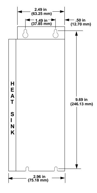
Figure 5-8: 500 W Narrow Drive (-DN) - Front View
