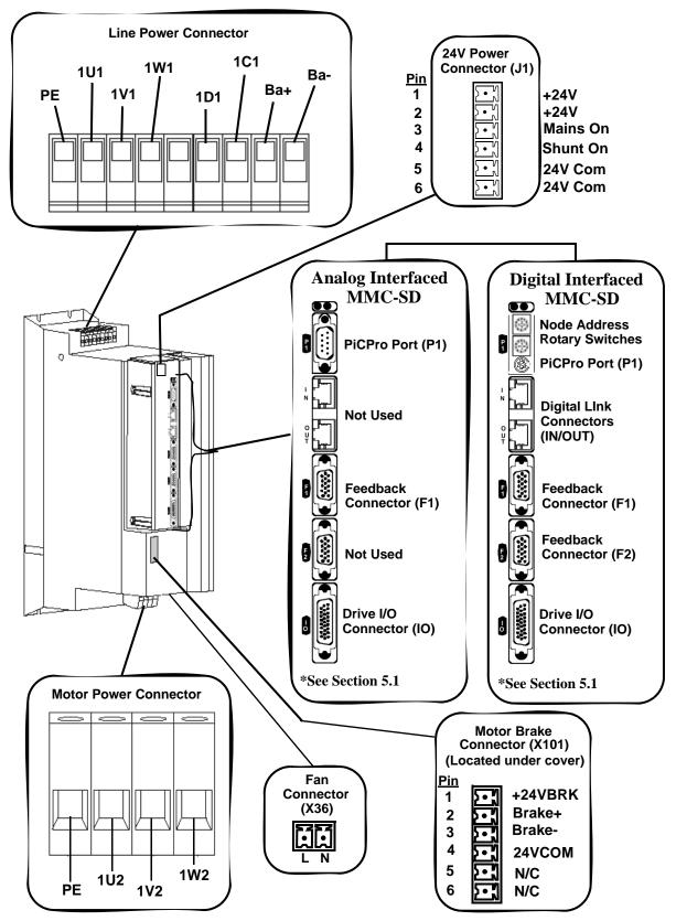
Figure 6-7: Connectors on the Size 4 460V Drive
