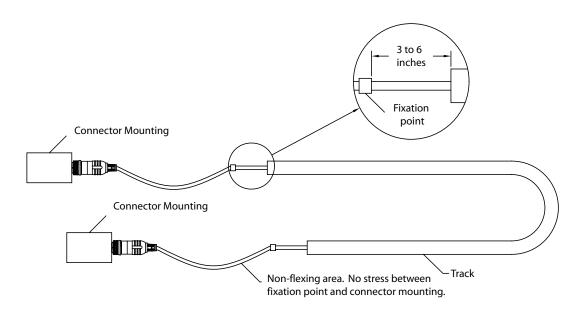
Observe the following precautions when installing flex cables:
