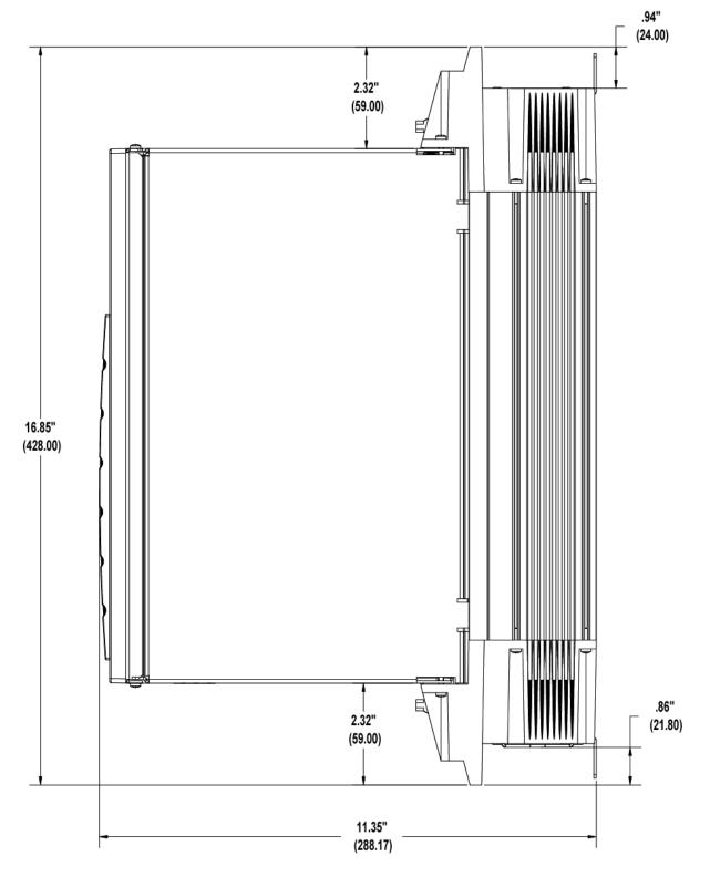
Figure 6-12: Size 2 460V Smart Drive - Side View
