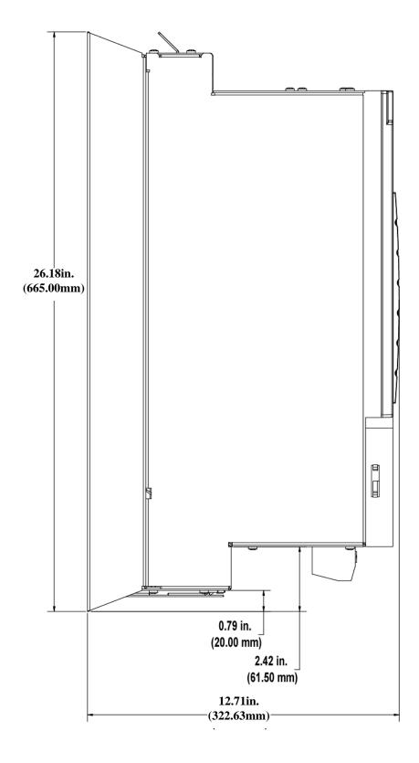
Figure 6-16: Size 4 460V Smart Drive - Side View
