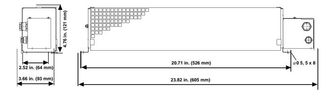
Figure 4-4: Mounting Dimensions for 460V External Shunt (P/N M.1302.7049)
