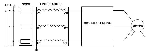
Line reactors are not necessary for the 230V MMC Smart Drives or the 460V size 1 and 2 MMC Smart Drives. Line reactors are required for the 460V size 3 and size 4 MMC Smart Drives.
