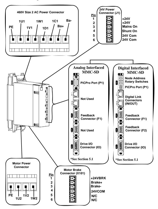
Figure 6-3: Connectors on the Size 2 460V Drive
