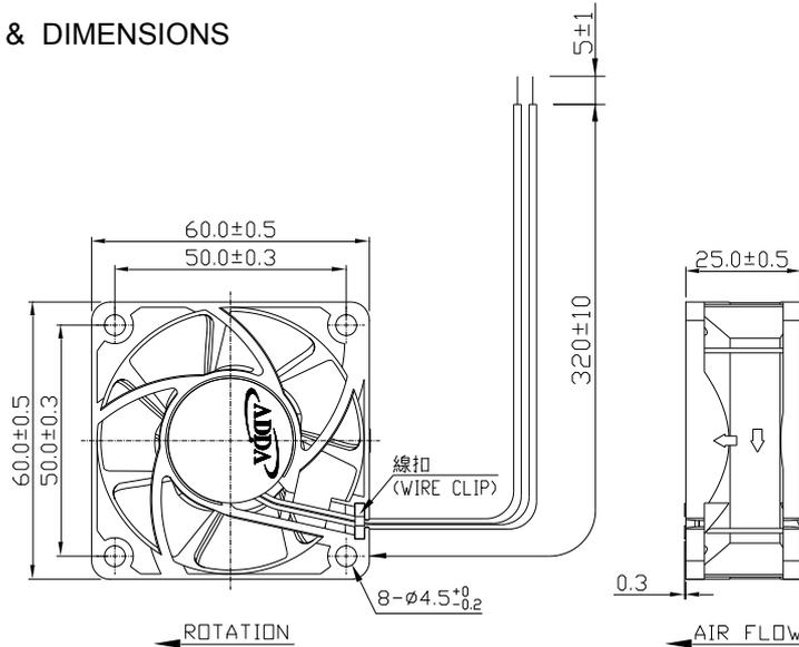
LEAD WIRES : UL 1007, AWG24 , L = 320 +/- 10 mm
