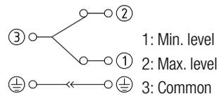
**Note:** to invert the contact status from NC to NO and vice versa, simply invert the float.
