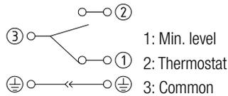
**Note:** to invert the contact status from NC to NO and vice versa, simply invert the float.
